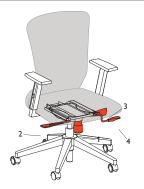
1. Tension Control Knob allows for greater spring tension control for a firmer or softer tilting motion. Turn counter-clockwise to increase tension, clockwise to decrease tension.
