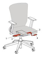
1. Tension Lever allows for greater spring tension control for a firmer or softer tilting motion. Push downward and back to increase tension, pull forward and up to decrease tension.
