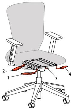
1. **Seat Height Adjustment** easily raises or lowers seat to desired height. To raise, lift weight off seat and pull upward on lever until seat reaches a comfortable height. To lower, lift upward on lever while seated and release to lock seat into desired position.
