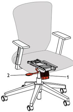
1. **Tension Control Knob** allows for greater spring tension control for a firmer or softer tilting motion. Turn counter-clockwise to increase tension, clockwise to decrease tension.
