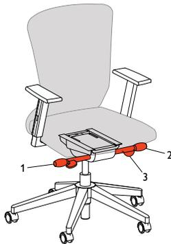
1. **Seat Height/Tension Control** easily raises or lowers seat to desired height and allows for more precise spring tension adjustment. To raise, simply lift weight off seat and pull upward on handle until seat reaches a comfortable height. To lower, lift upward on handle while seated and release to lock seat into desired position. To adjust tension for a firmer or softer tilting motion, turn knob counterclockwise to increase tension, clockwise to decrease tension.
