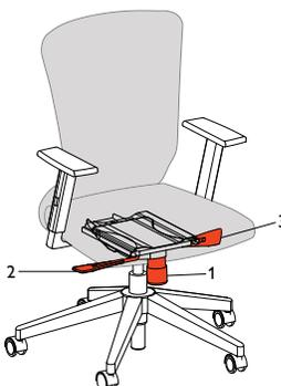
1. **Tension Control Knob** allows for greater spring tension control for a firmer or softer tilting motion. Turn counter-clockwise to increase tension, clockwise to decrease tension.
