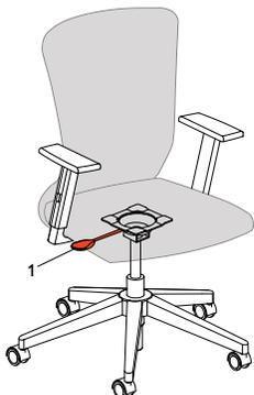
1. **Seat Height Adjustment** easily raises or lowers seat to desired height. To raise, lift weight off seat and pull upward on lever until seat reaches a comfortable height. To lower, lift upward on lever while seated and release to lock seat into desired position.
