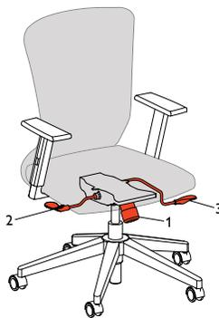
1. **Tension Control Knob** allows for greater spring tension control for a firmer or softer tilting motion. Turn counter-clockwise to increase tension, clockwise to decrease tension.
